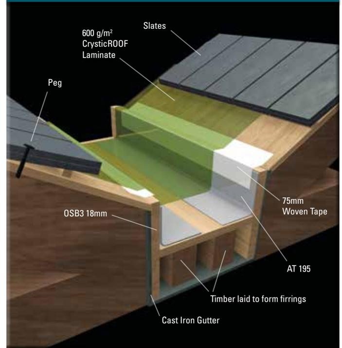
In order to kick the stone slates up, a full board will need to be laid along the pitched roof with the batten nailed in place.
