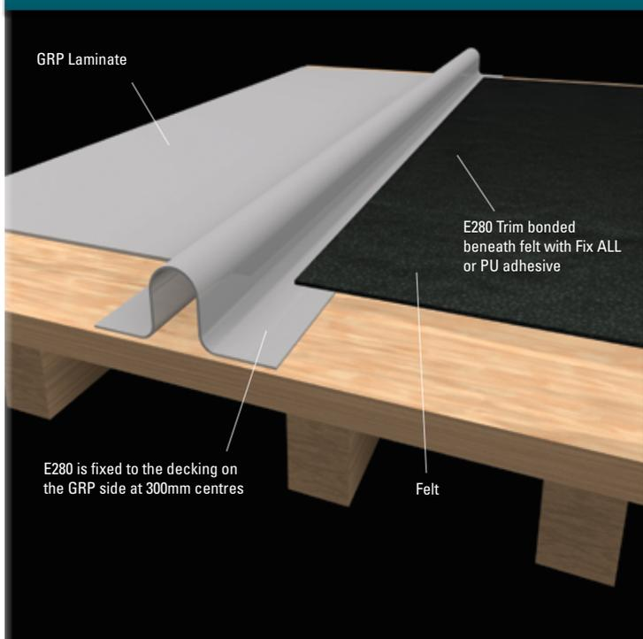
Not only is the E280 compatible with C5 closures, but it can be used for creating rolls on any ridge details, expansion joints on large roofs (50m<sup>2</sup> or over) or to bridge GRP to felt roofs.
