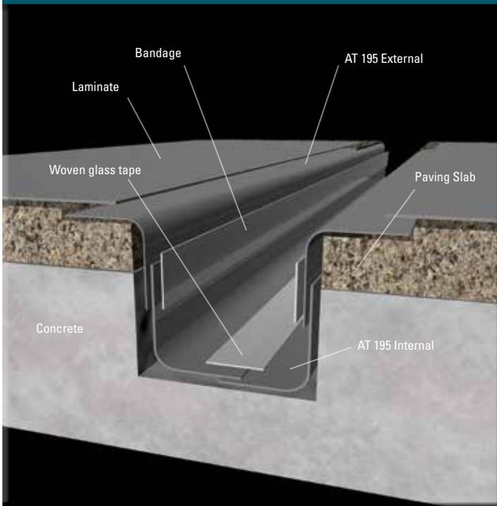
Wherever laminate is used to cover an area which runs parallel to another laminate surface, AT195 Internal and External trim is recommended.
