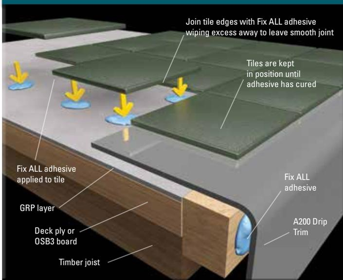
Once the GRP roof has fully cured, tiles can be applied. Preferably tiles should be laid as soon as the roof has cured with any dirt and debris being removed from the roof. If the roof has been left for any length of time and surface dirt and debris have accumulated, it will be necessary to thoroughly clean the surface. It is strongly recommended that a light sanding and surface wipe with Acetone be used to ensure the best possible adherence.
