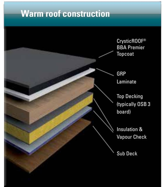
GRP roofs can be used easily to meet either a cold or a warm roof specification. When working with a warm roof, the first step will be to apply a sub-deck to the joists at 300mm centres, followed by a vapour check and laying an insulation sheet over the top. You can also buy insulation sheets with a vapour check in-situ.
