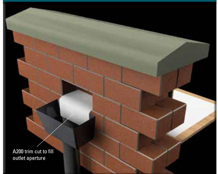
It is recommended that the pre-formed GRP outlet lining is constructed at the same time as the trims are fixed to the roof. It is possible for two D260s to be joined together using the woven glass tape in order to seal the joint after the trims have been securely fixed to the decking using clout nails.
